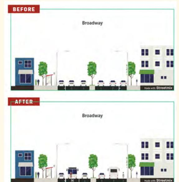
Broadway cross-section before (top) and after (bottom) bus lanes were installed.
