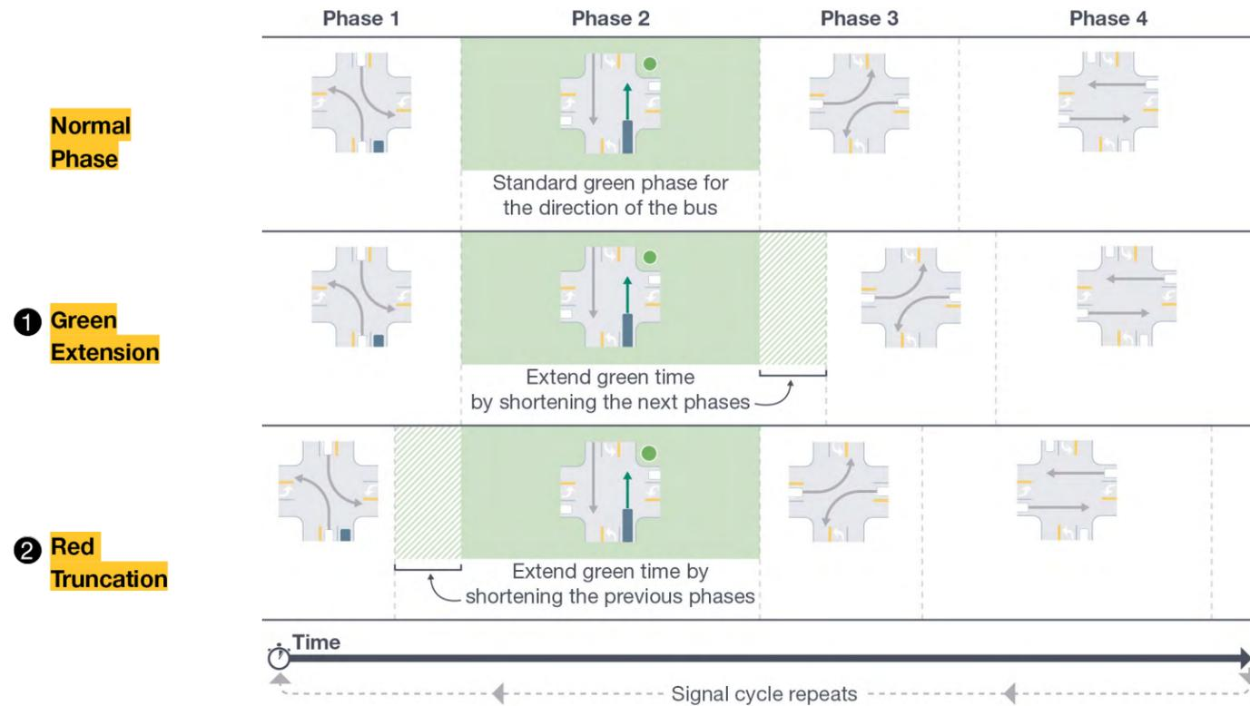
Note: Signal phase diagrams are schematic only to demonstrate the functionality of TSP strategies at a high level. Exact times and phase changes will vary.
