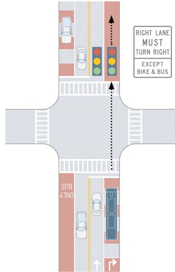
**2 Bus Operating in a Shared Bus Lane with Right Turns with the Bus Traveling through the Intersection**
